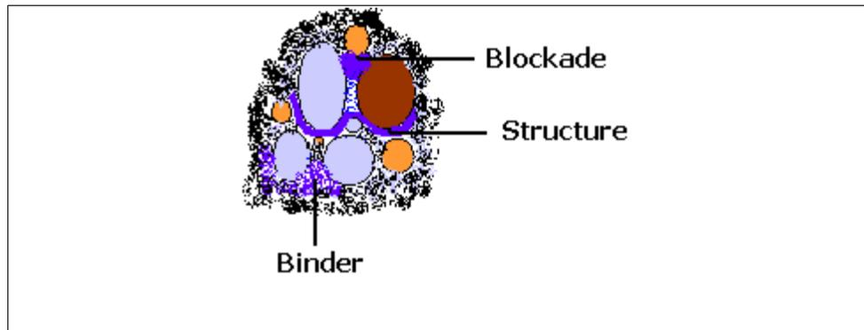
**Figure 1.** *Effect of the plastic inside an asphalt mixture*
