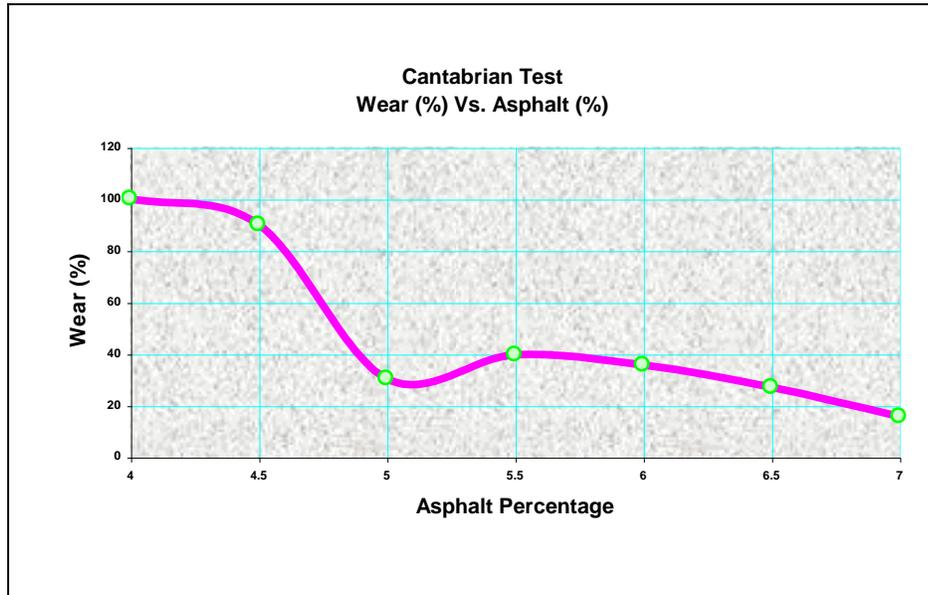
Graph 1. Optimum Percentage of Asphalt obtained with the Cantabrian Method
