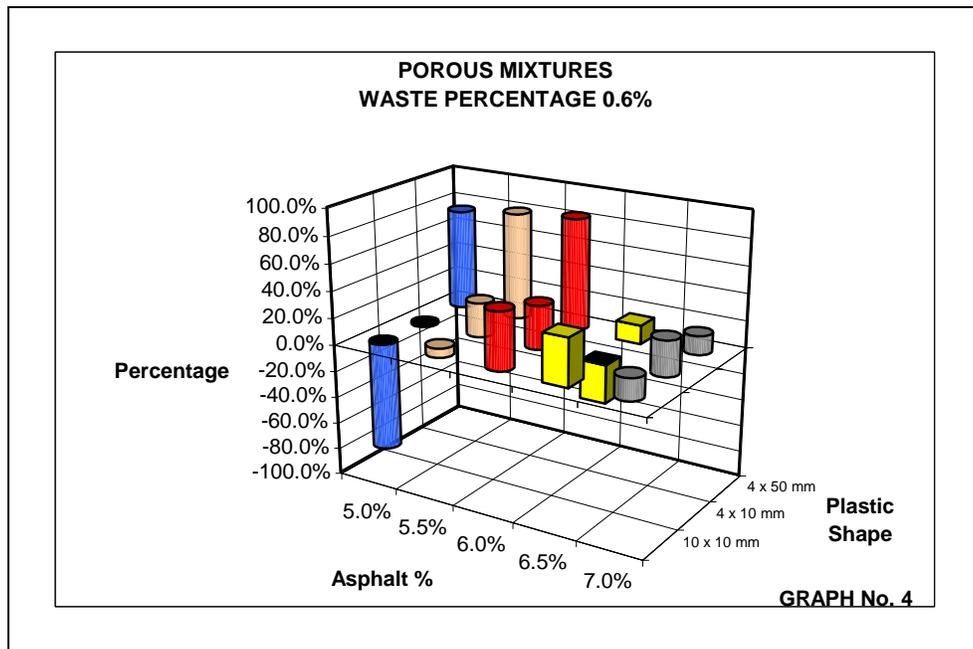
**Graph 4.** Relationship between Plastic Shape, Asphalt Percentage and mechanical properties with 0.6% of Waste
