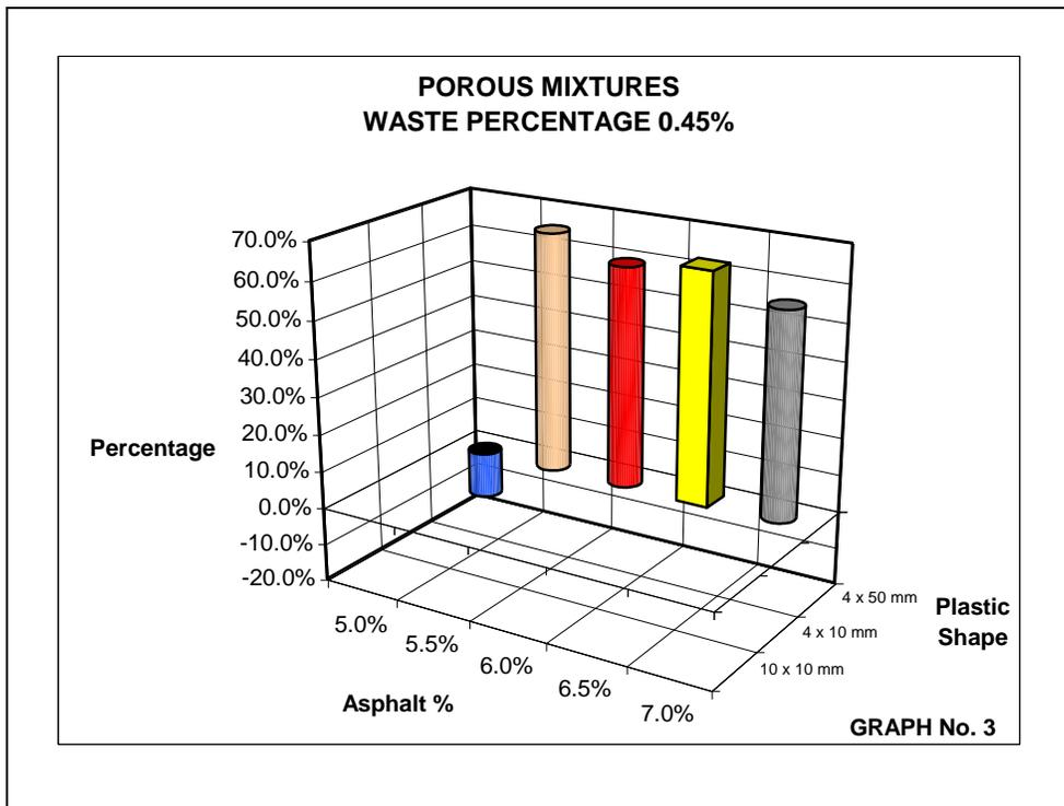
**Graph 3.** Relationship between Plastic Shape, Asphalt Percentage and mechanical properties with 0.45% of Waste
