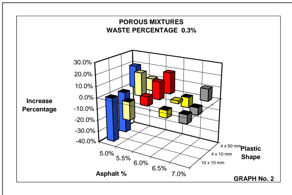
**Graph 2.** Relationship between Plastic inclusion shape, Asphalt Percentage and mechanical properties with 0.3% of Plastic Waste.
